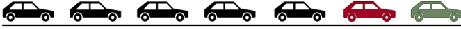
Fig. 5. Vehicle formation used in simulation. A trajectory leader (in green) driving a speed profile drawn from the dataset is placed in front of a CAV (in red) which is followed by a platoon of 5 human vehicles (in black), modeled using the Intelligent Driver Model.
